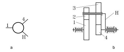
Figure 1. 2DOF planetary unit: a – symbolical scheme, b – structural scheme;
