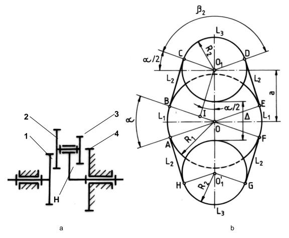
Figure 2: Planetary belt (chain) transmission structural scheme (a) and dimensions (b) {2}
