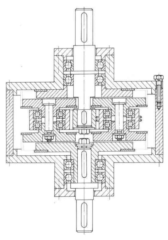
Figure 3. Assemble drawing of belt planetary transmission [2]
